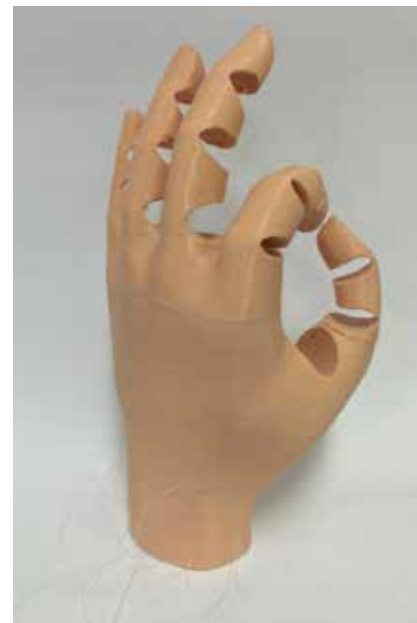
The left two images are parametric models of rendered hands. The image on the far right is the 3D printed version of the model with a series of fine tendon cables attached.
