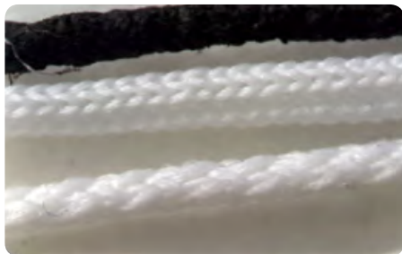
Figure 6: Knitting structure coated with conducting polymer for use as a textile sensor.
