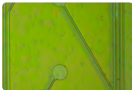
Metal electrodes patterned on polyimide developed through the Australian National Fabrication Facility (ANFF).
