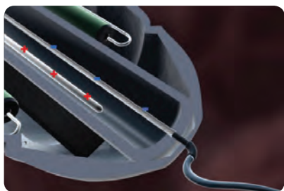
Image shows the tail region and insides of futuristic microbot with the flagella-like tail rotated by a length of the research team's new carbon nanotube yarn torsional muscles.
